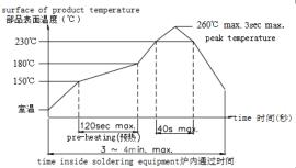
9 Automatic Flow Soldering (自动焊接)
