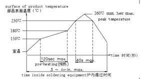
Automatic Flow Soldering (自动焊接)
